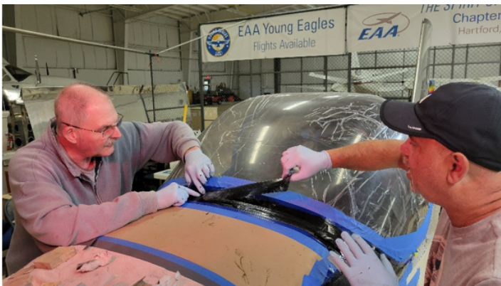
Mark and Steve laying fiberglass strips to fabricate the canopy fairing.
