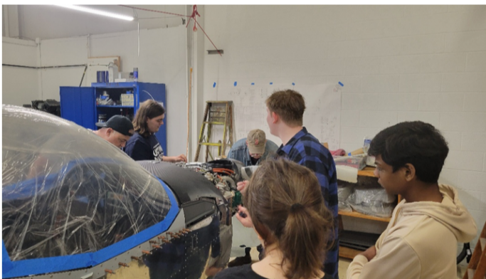
Build team members installing the lower cowling with cooling baffle attached.
