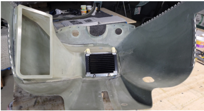
Lower Cowl with Cooling Baffle permanently attached.
