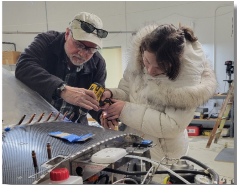
Fabrizia (right) match drilling attachment holes through the canopy into the forward bow while assisted by Rick. Photo Credit: Joe Kline
