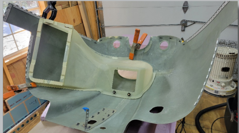
Cooling Baffle clamped to lower Cowling
