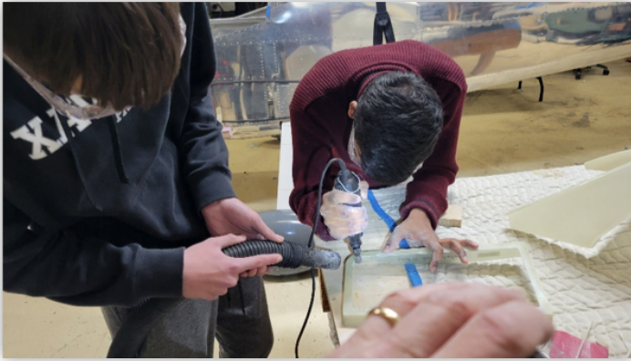
Trevor Snow (Left) and Pugal Prabha trimming the Cooling Baffle
