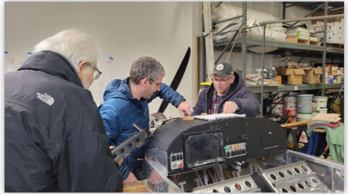
Ron Jones (Left) installing the radiator while Dave Trenkner (Center) and Joe Kline (Right) work to install an Adel Clamp on the Throttle and Choke Cables
