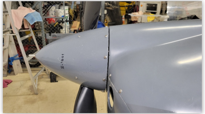
The fit between the cowling and the spinner. The team was very happy with how well the installation was performed.
