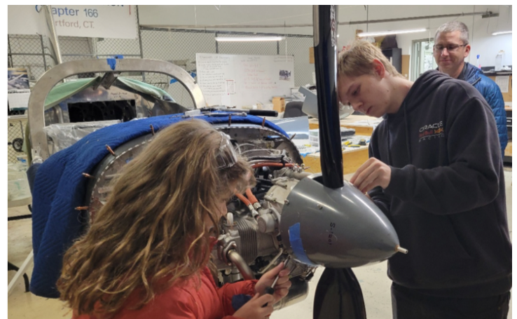
(left) Nate and Aaron counter sinking holes in the upper cowl in preparation for hinge installation. (right) Kai and Jackson installing the mounting screws for the spinner after having installed the nut-plates with rivets.
