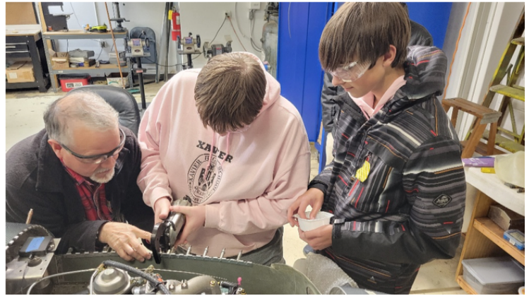
Rick teaching Ryan and Trevor how to use a pneumatic squeezer to install rivets on the lower cowl hinge. (Photo credit Josh Snow)
