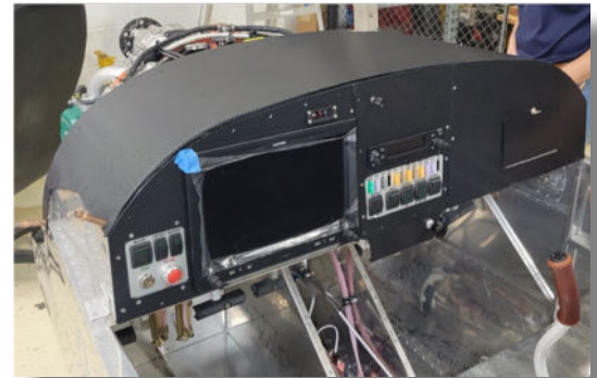
Initial start-up of G3X Touch Primary Flight Display and the carbon fiber vinyl wrapped panel
