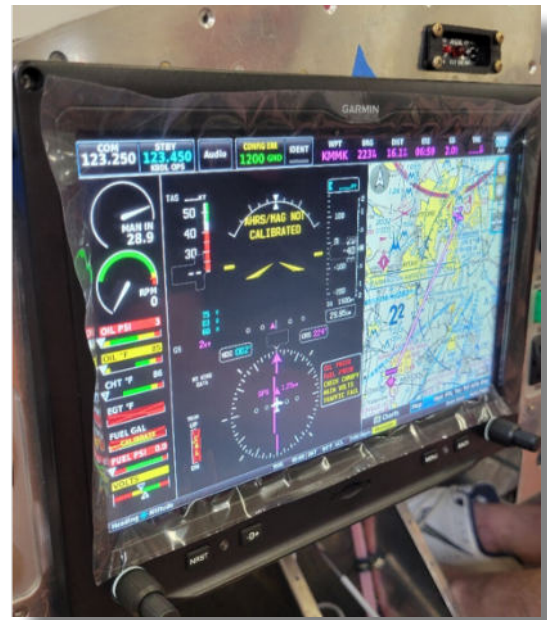
Initial start-up of G3X Touch Primary Flight Display and the carbon fiber vinyl wrapped panel
