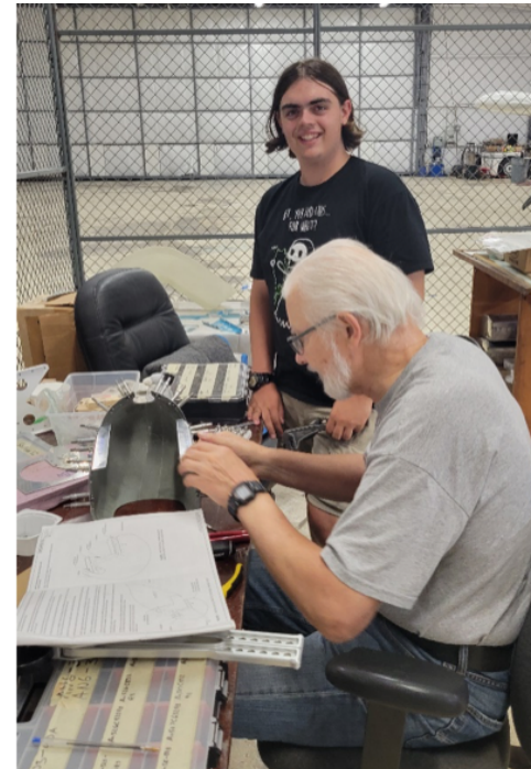
Seth and Ron (seated) assembling the Nose Wheel Fairing Credit: Rick Montero
