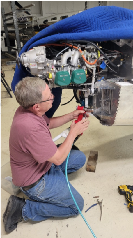
Kline (new member) riveting the Cooler Door Assembly to the Firewall Credit: Rick Montero
