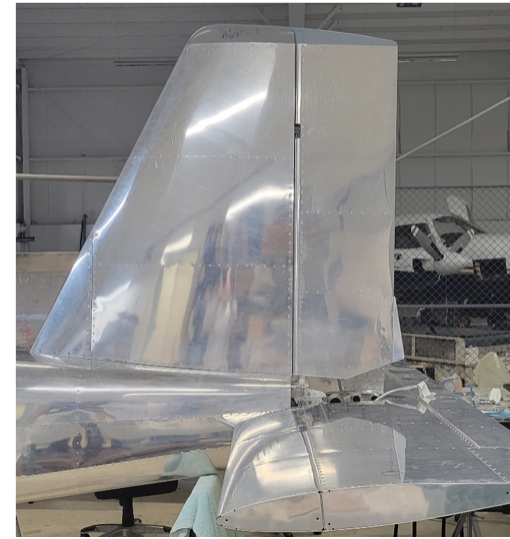
Vertical Stabilizer and Rudder Fairings mounted to the empennage of the RV-12
