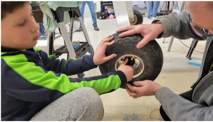
Left: Jude Murphy installing the main wheel axle nut under the guidance of Mark Welch. Right: Main gear axle and shim installed to correct a Toe-in condition.
