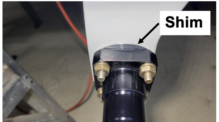
Left: Jude Murphy installing the main wheel axle nut under the guidance of Mark Welch. Right: Main gear axle and shim installed to correct a Toe-in condition.
