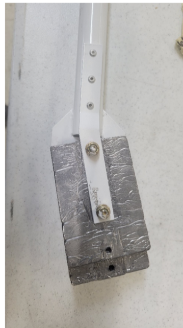
Left: showing service bulletin (SB-00067) modifications made to the Stabilator Counterbalance Arm to add reinforcing straps that help prevent fatigue failure. Right: Magnetometer (arrow) installed within the tailcone.
