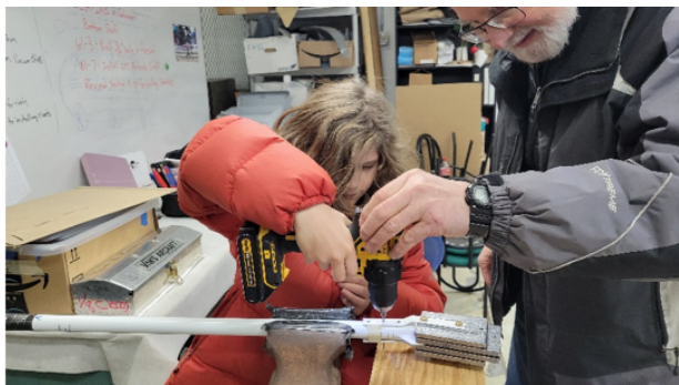
Kai Trenkner match drilling rivet holes in the stabilator counterbalance arm while being guided by Ron Jones. This modification was required by Service Bulletin SB-00067.
