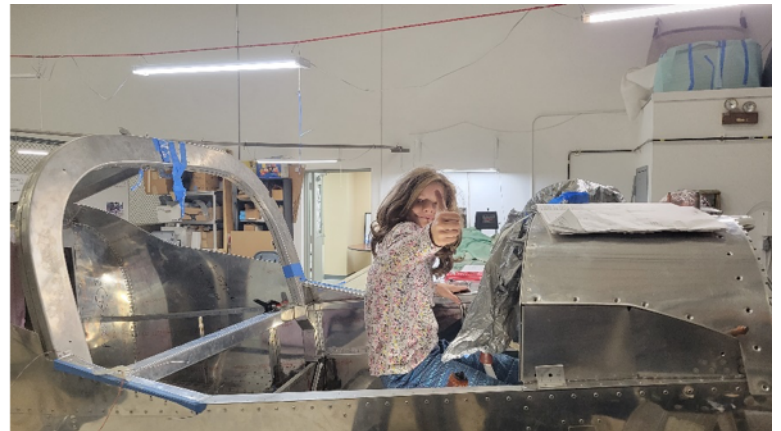
(above) Kai Trenkner testing the pedal cable connections to the Rudder. Photo Credit: Rick Montero
