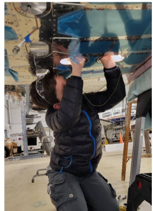
(above right) Jude Murphy adjusting the turnbuckles on the stabilator cables and installing the locking spring clips. This procedure is more easily accomplished by someone with small hands and excellent vision. Photo Credit: Rick Montero
