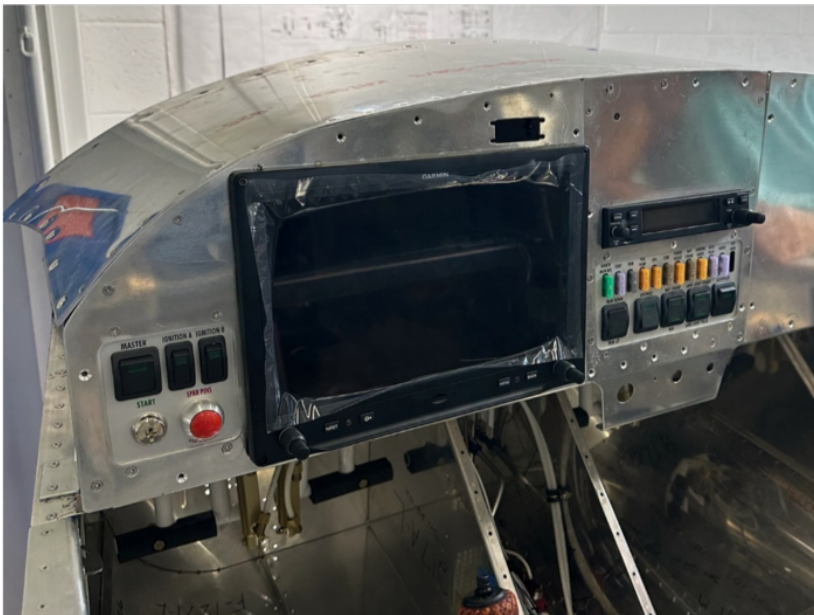
The Ignition Module, G3X Touch PFD, Power/Switch module and Com Radio installed in the Instrument Panel. Photo Credit: Mark Welch.
