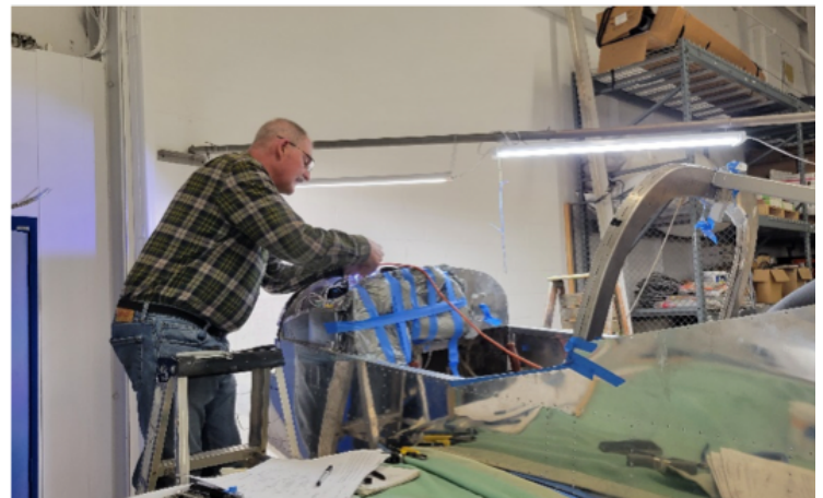
Photo of Mark Welch making the final connections in the avionics wiring harness.
