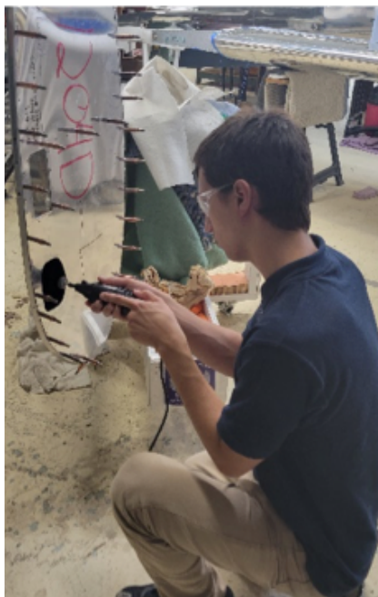
Will Coates shown deburring the access hole in the left wing closeout panel. Photo credit: Rick Montero
