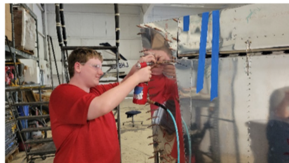
Ryan Coughlin shown riveting the closeout panel to the left wing. Photo Credit: Rick Montero.
