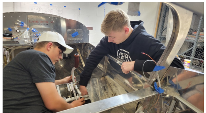
Seth Varroto (L) and Noah Foster (R) shown attaching the push rods between the control sticks and the flaperon bell crank.
