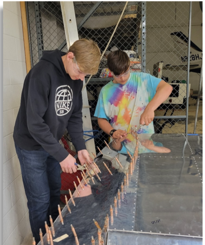
Noah Foster (L) and Seth Varroto (R) attaching the wing tip close out panel to the right wing. Photo Credit: Rick Montero.
