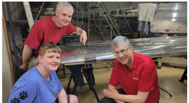
Ryan Coughlin (left foreground), Mike Coughlin (left rear) and Ken Katz (right) shown next to landing light lens clecoed into the right wing after it was trimmed to size. Photo Credit: Rick Montero.
