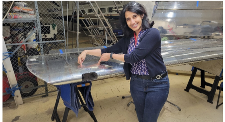
Manu Ramesh pointing toward the opening cut into the leading edge of the right wing and the matched drilled holes for the landing light lens. Photo Credit: Rick Montero.
