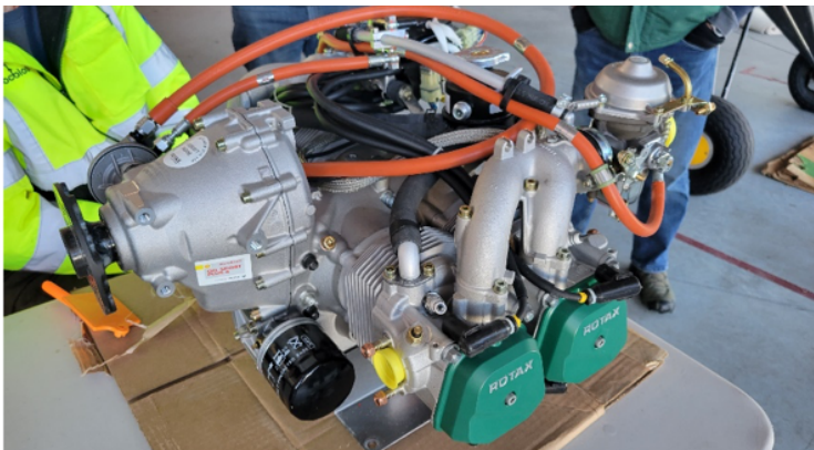
The Rotax 912 engine following cylinder inspection (left) and wiring in process (right). Photo Credit: Rick Montero and Larry Anglisano.
