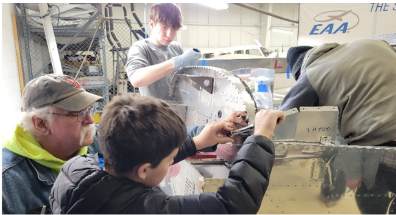
Ed Semeneshen (left) teaching Jude Murphy (lower center) how to torque the bolts for the Brake Fluid Reservoir. Parker Glaude (upper center) is removing residual RTV sealant while Steve Oakley (far right) is installing the wiring harness, Photo Credit: Rick Montero
