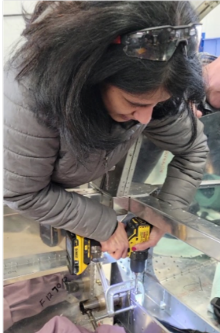
Manu Ramesh drilling a slide channel into the landing gear beam. Photo Credit: Rick Montero
