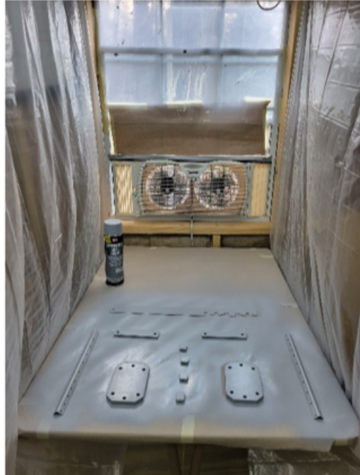
Service Bulletin parts being primed in Rick Montero's workshop. Photo Credit: Rick Montero
