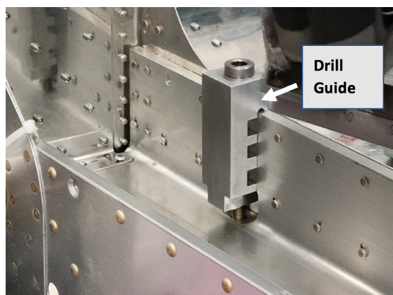
Drill guide in position to create a side channel in Landing Gear Beam. Photo Credit: Rick Montero
