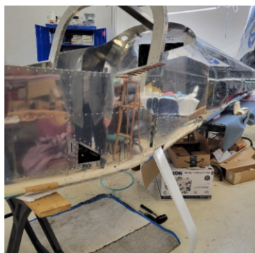
Left Landing Gear Leg installed following Service Bulletin Upgrade. Photo Credit: Rick Montero
