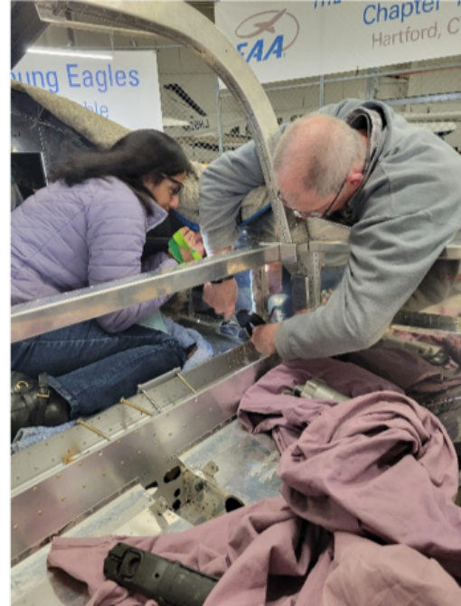
Manu and Mark Welch installing rivets between Baggage Area Skin and Landing Gear Beam. Photo Credit: Rick Montero
