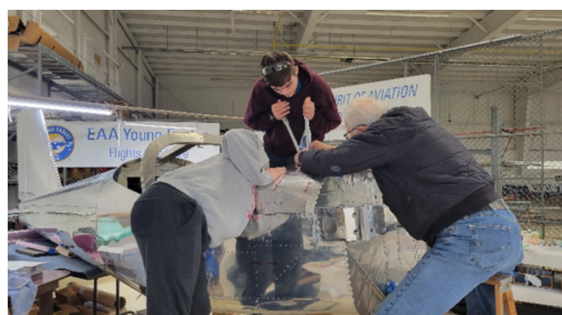
Photo showing Mitch Rathbone, Seth Verratto, and Ron Jones installing the upper fuselage skin. Photo Credit: Rick Montero
