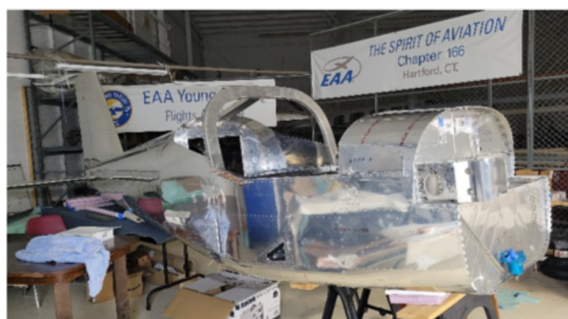
Photo showing side view of upper forward fuselage installed. Photo Credit: Rick Montero
