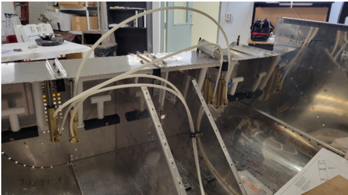
Rudder Pedals, Master Cylinders and Brake Lines installed in Fuselage. Photo Credit: Rick Montero.
