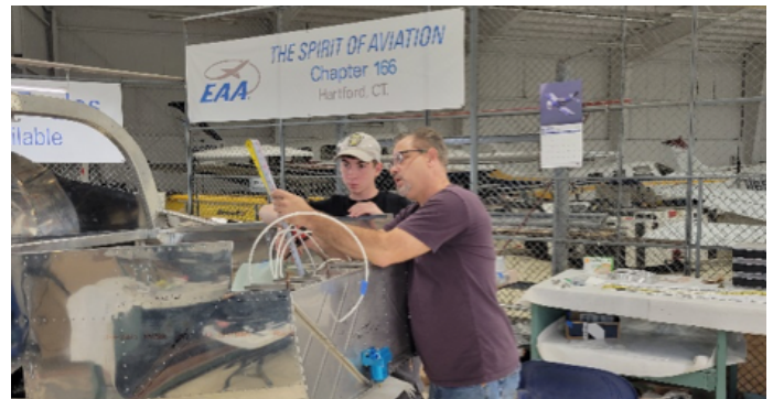
Photo showing Steve Oakly (R) and Parker Glaude (L) measuring fuel line in just prior to installation. Photo Credit: Rick Montero.
