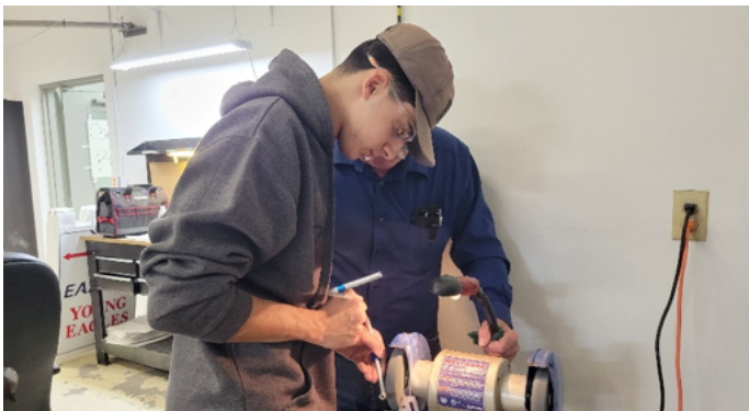
Logan Vidal deburring fuel line. Photo Credit: Rick Montero.
