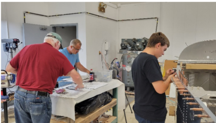
Photo showing Ed Semeneshen (L) and Steve Oakley (M) working on the Baggage Bulkhead and Seth Varrato (R) installing the Fuselage Vent Doors. Photo Credit: R. Montero
