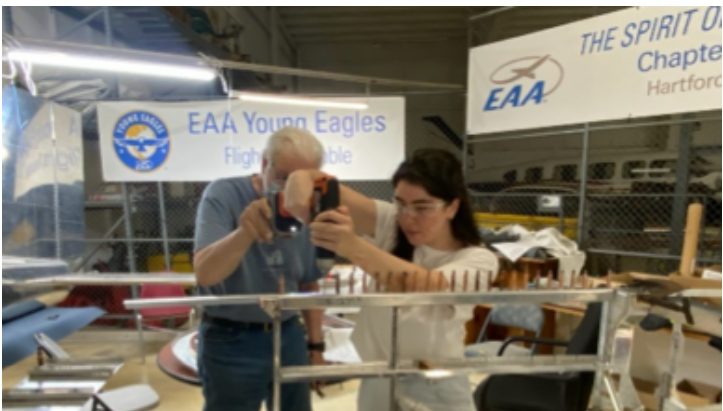
Lauryn Santino (R) and Ron Jones (L) match drilling the canopy desk to the longeron. Photo credit: S. Oakley
