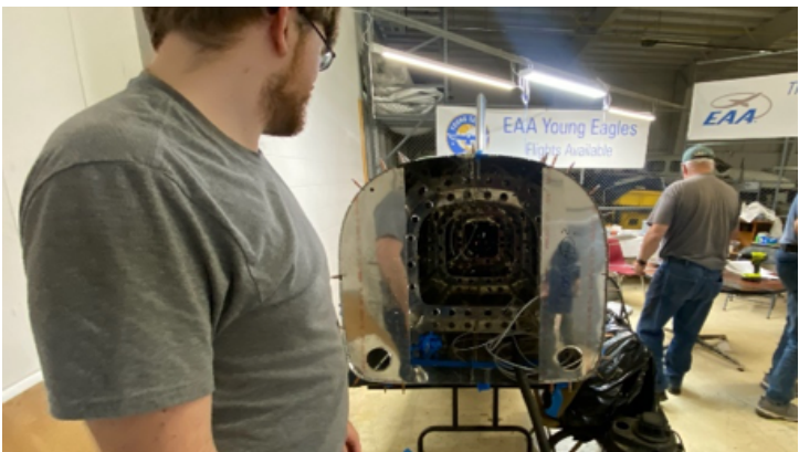
Ludwig Johanning checking the fit of the Baggage Bulkhead Panels to the Tailcone. Photo credit: S. Oakley
