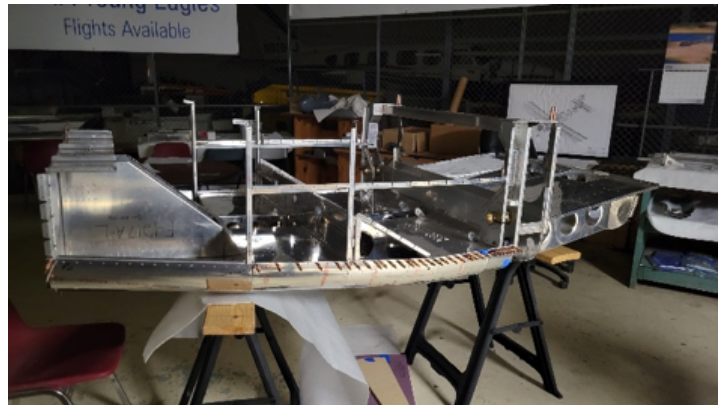
Firewall (L) and Mid-Fuselage assembly. Photo credit: R. Montero
