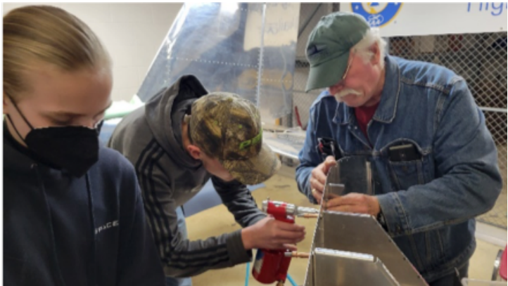
Sing Cohn (L) and Austin Fuoco (C) riveting the corner skins onto the lower Firewall assembly with guidance from Ed Semeneshen. credit: R. Montero
