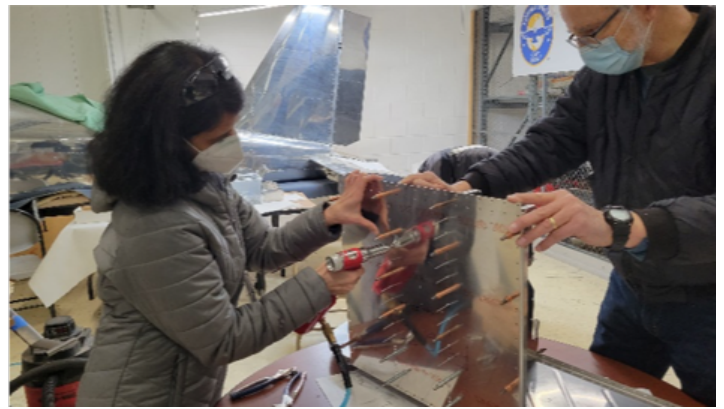
Photo showing Manu (L) riveting the Firewall Bottom Panel to the Tunnel Ribs while Ron (R) supports the assembly. Photo credit: R. Montero
