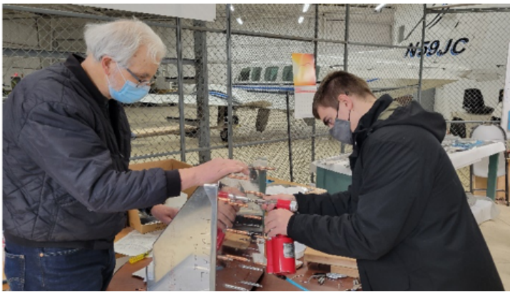
Photo showing Seth (R) riveting the Firewall Bottom Panel to the Tunnel Ribs while Ron (L) supports the assembly. Photo credit: R. Montero
