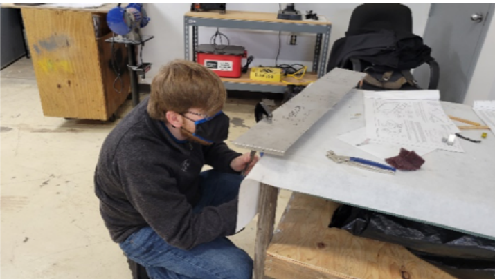
Photo showing Ludwig riveting nut plates to the Firewall Shelf. Photo credit: R. Montero
